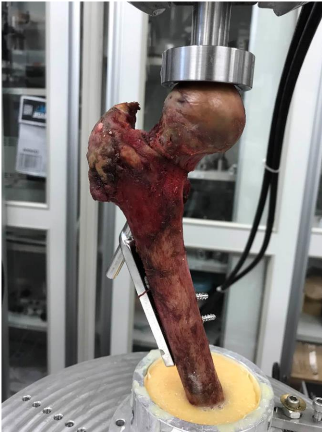
Experimental setup for a whole femur with an metallic implant
